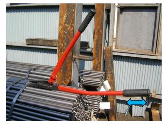
•As for the conventional product for steel Strap Cutter, it is necessary to hit the end of handle by Hammer, for biting the blade of Steel Strap. However, our new product, SS 600-SS includes Hammer function (Sliding Stricker).
